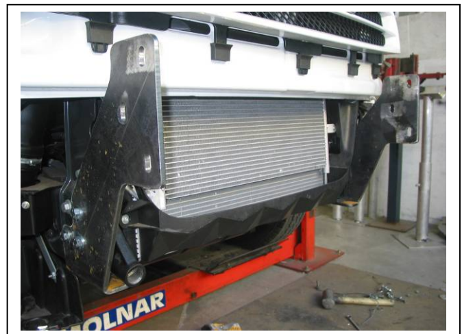
Figure 3: ECB Steel mounting system fitted
