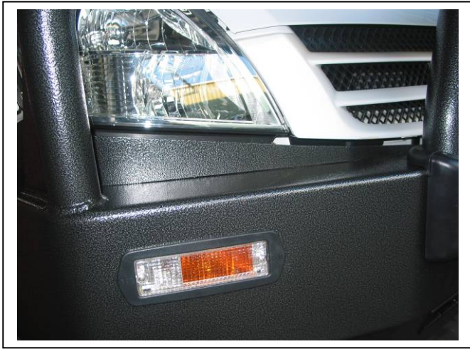
Figure 6: Adjust infill to suit light and guard shape
