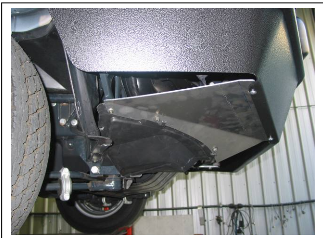
Figure 10: Drivers side splash panel extension.
