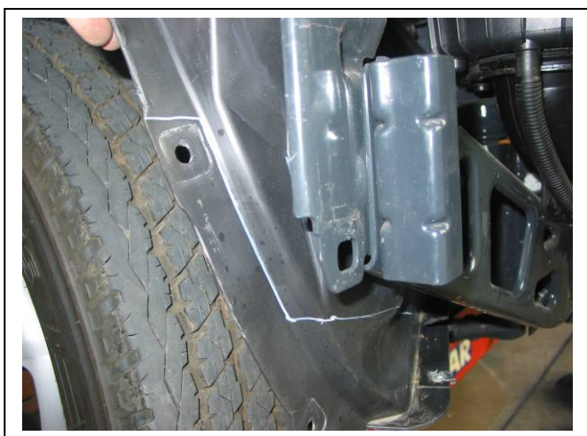
Figure 4: Marking inner guard for trim using bumper support as guide
